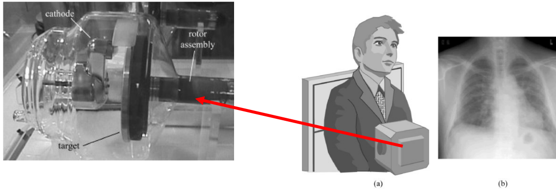
Figure 1.1 Illustration of conventional x ray. (a) Acquisition setup and (b) example of a chest study.
